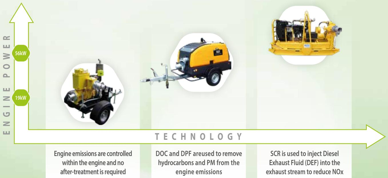
**THIS GRAPH ILLUSTRATES HOW EMISSION CONTROL TECHNOLOGY CHANGES ACCORDING TO THE ENGINE POWER RANGE.**
